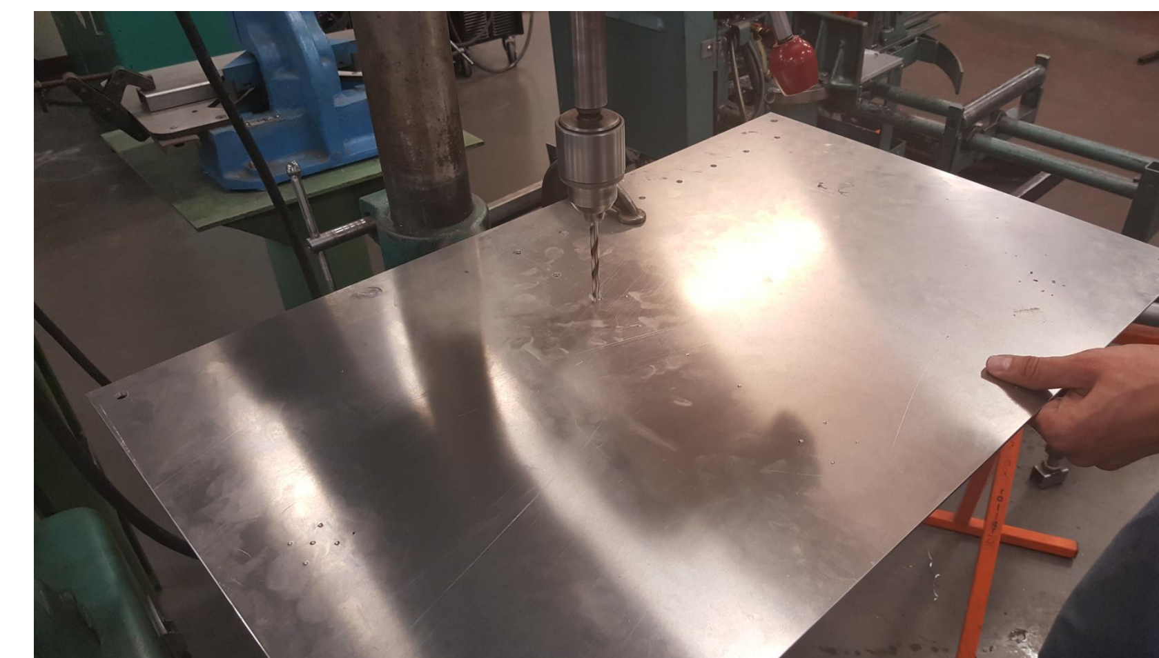
Figure 2: Drilling of Aluminum Sheet Metal
