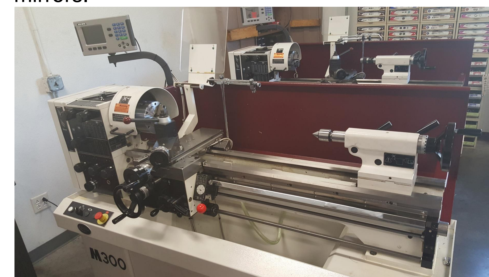
Figure 3: Turning Lathe for Aluminum Billets
